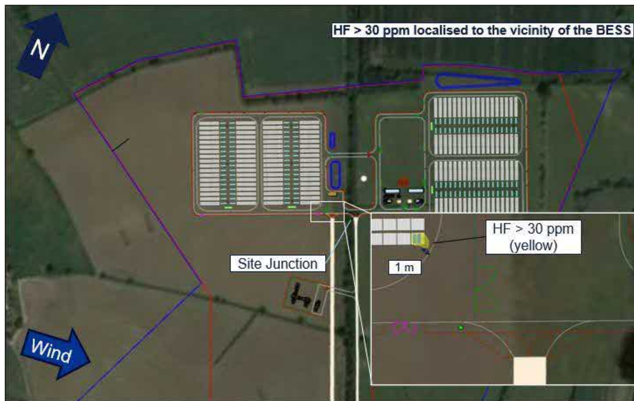
Figure A 2: Case 102 –Hydrogen Fluoride Plot with Wind from W at 8.5 m/s
