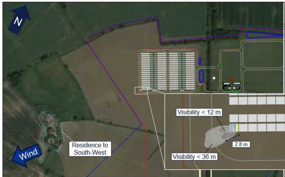
Figure A 15: Case 103 –Visibility Plot with Wind from NE at 5 m/s
