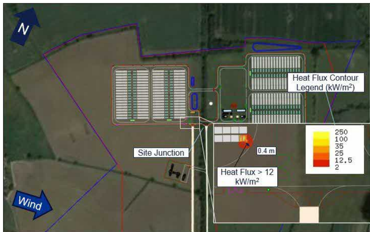
Figure A 10: Case 102 –Heat Flux Plot with Wind from W at 8.5 m/s
