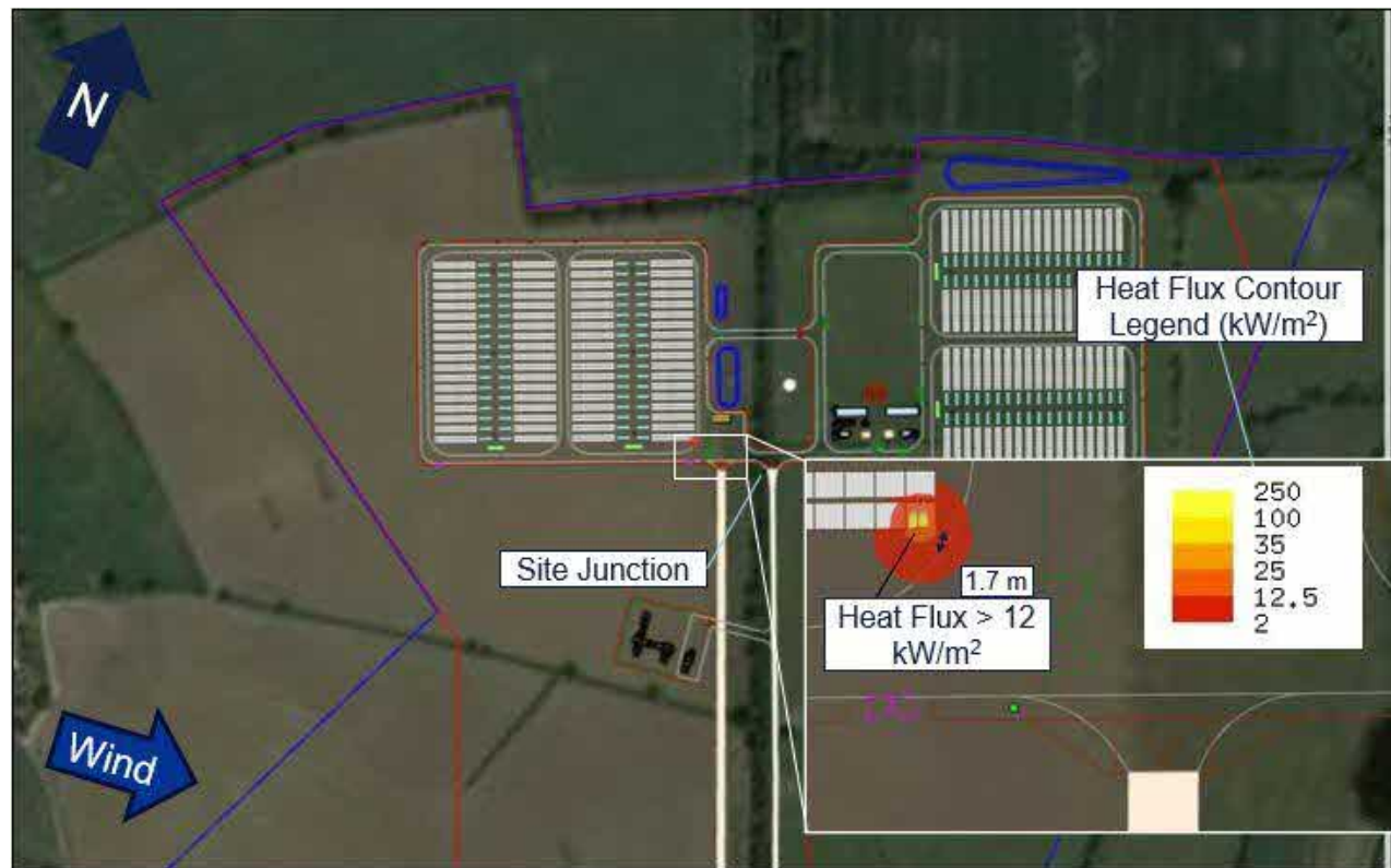
Figure A 9: Case 101 –Heat Flux Plot with Wind from W at 5 m/s
