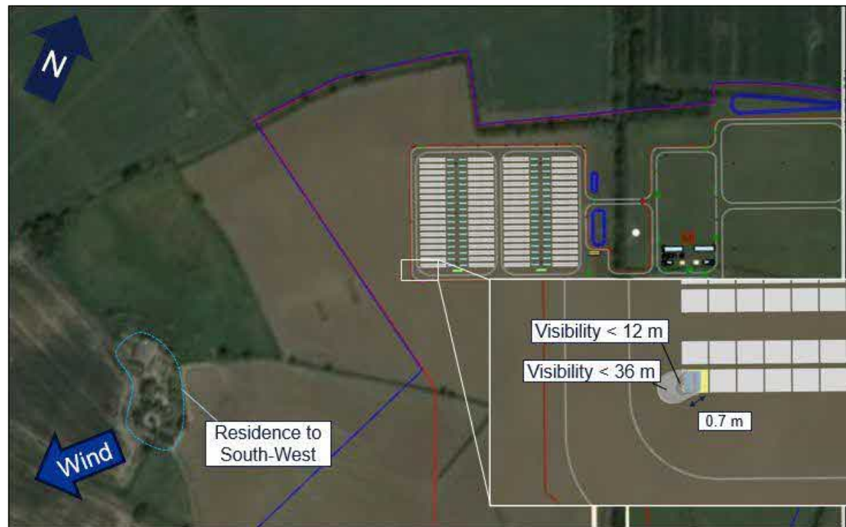
Figure A 16: Case 104 –Visibility Plot with Wind from NE at 8.5 m/s
