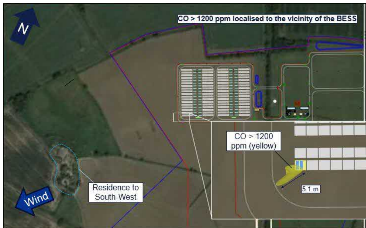
Figure A 7: Case 103 –Carbon Monoxide Plot with Wind from NE at 5 m/s
