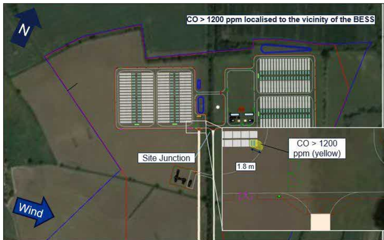
Figure A 6: Case 102 –Carbon Monoxide Plot with Wind from W at 8.5 m/s
