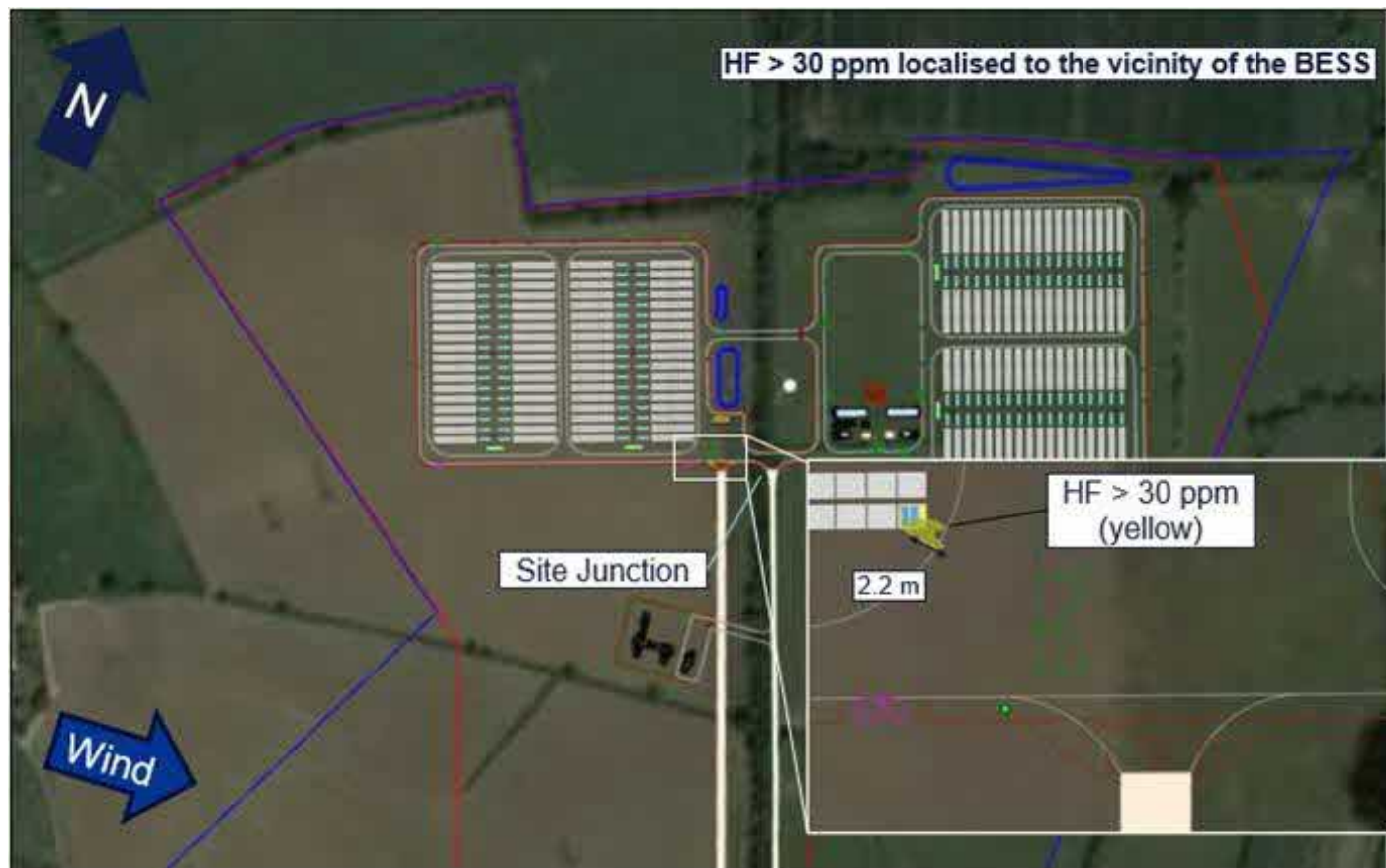
Figure A 1: Case 101 –Hydrogen Fluoride Plot with Wind from W at 5 m/s
