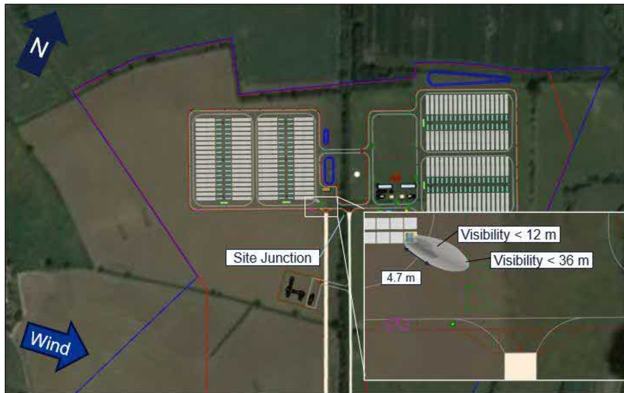
Figure A 13: Case 101 –Visibility Plot with Wind from W at 5 m/s
