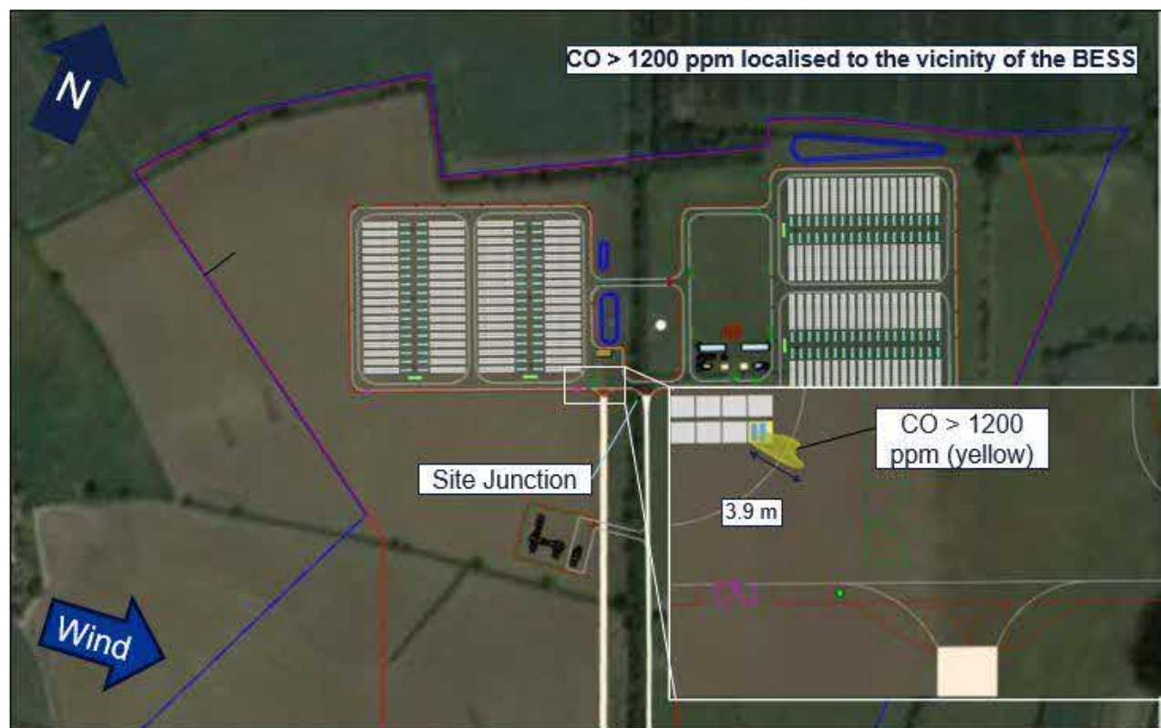
Figure A 5: Case 101 –Carbon Monoxide Plot with Wind from W at 5 m/s
