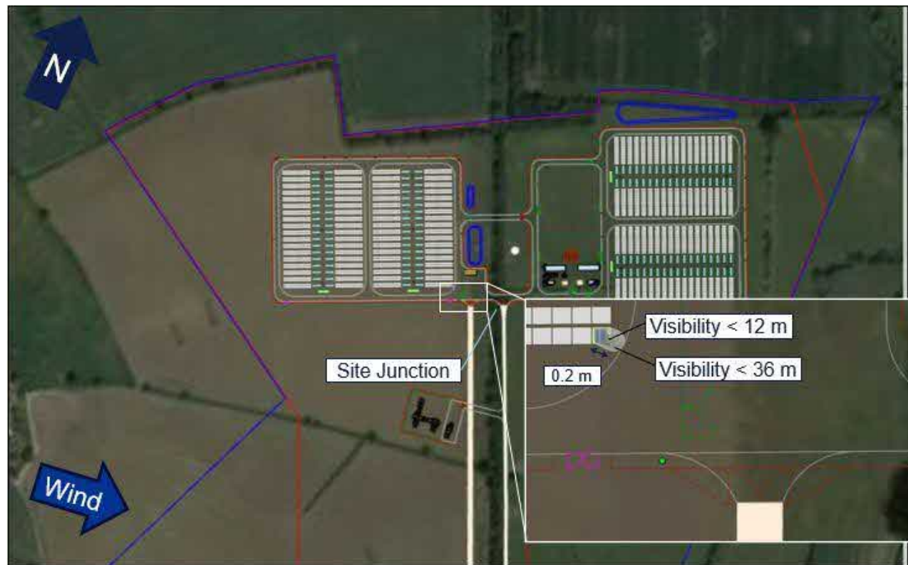
Figure A 14: Case 102 – Visibility Plot with Wind from W at 8.5 m/s
