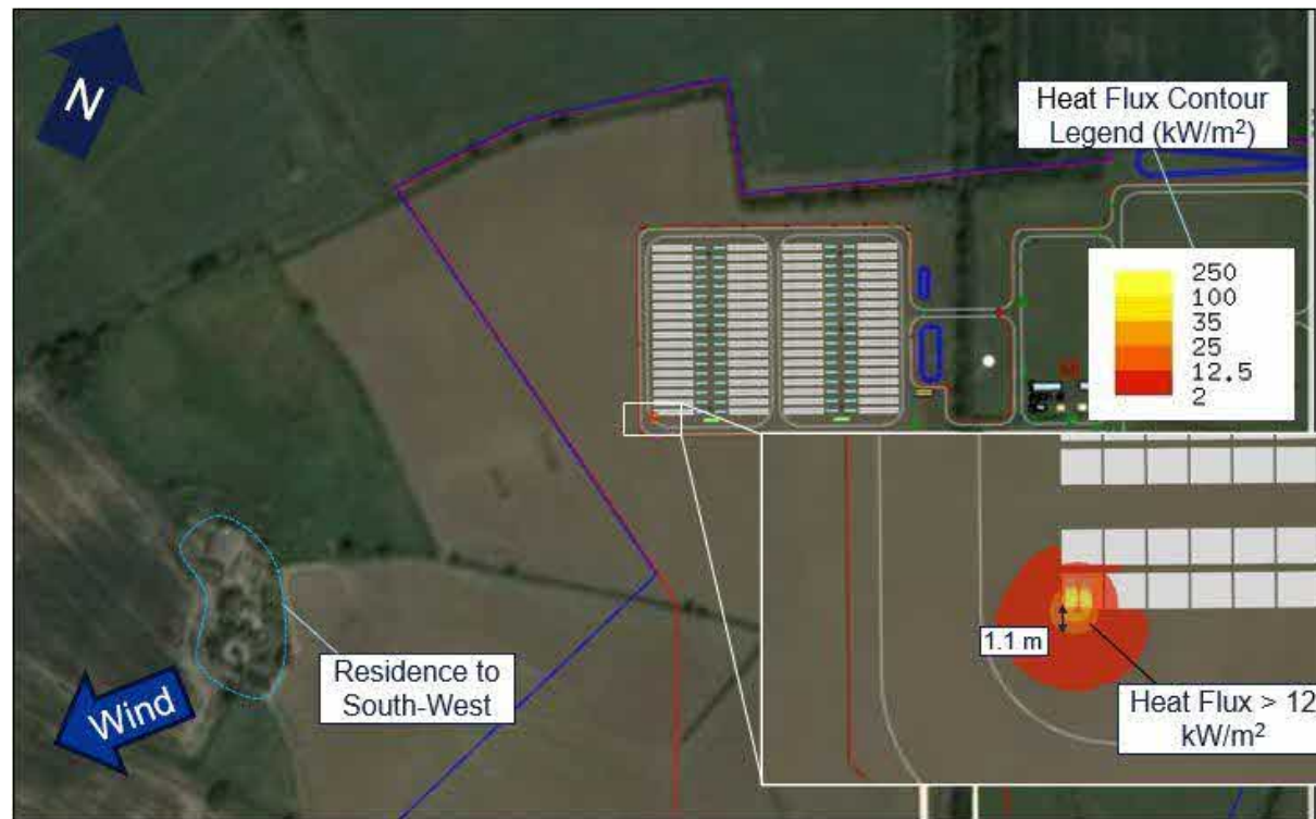
Figure A 11: Case 103 –Heat Flux Plot with Wind from NE at 5 m/s
