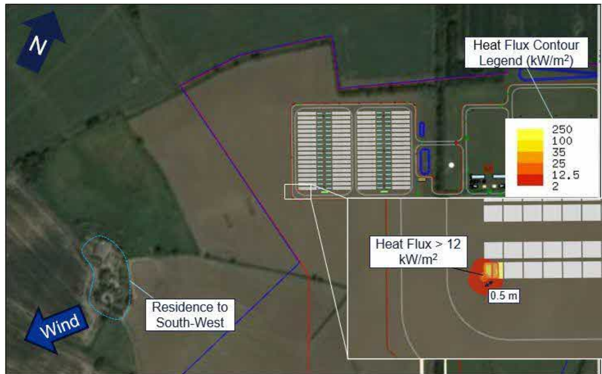
Figure A 12: Case 104 –Heat Flux Plot with Wind from NE at 8.5 m/s
