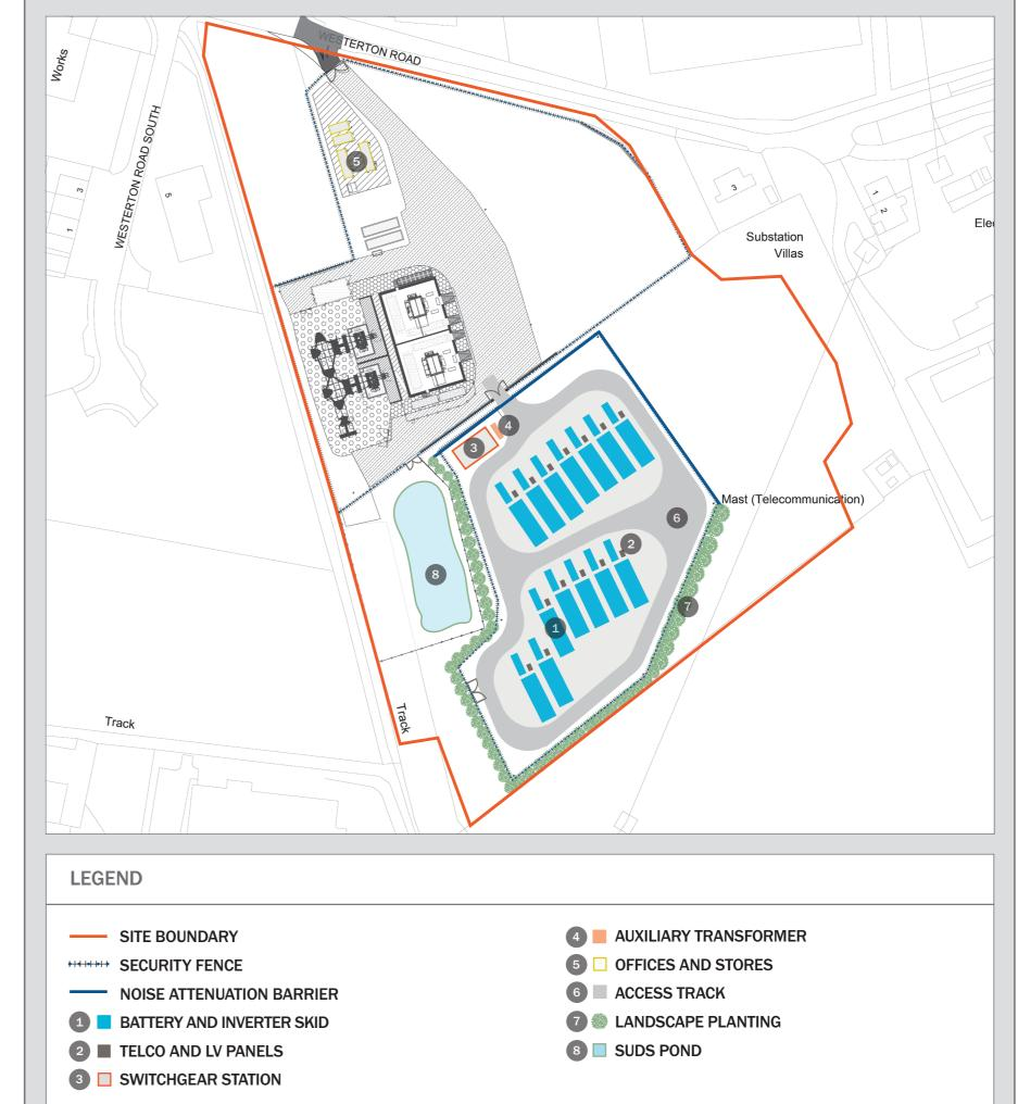
In 2020, Statkraft received planning consent for Keith Greener Grid Park development, this included 19.9MW of battery storage and two synchronous compensators. The batteries were not built but the synchronous compensators have been operational since 2022.
