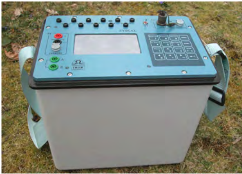
SYSCAL Pro Switch-48 unit with its graphic LCD screen
