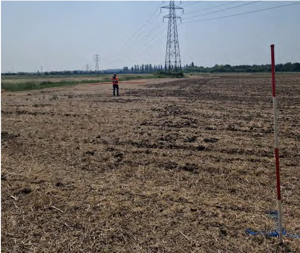
Plate 4: Data acquisition using the CMD system at the site (Field 12 looking north)
