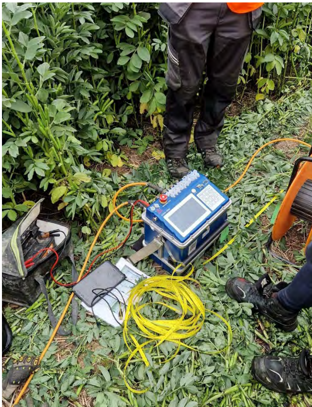
Plate 5. Data acquisition using the Syscal system in Field 9
