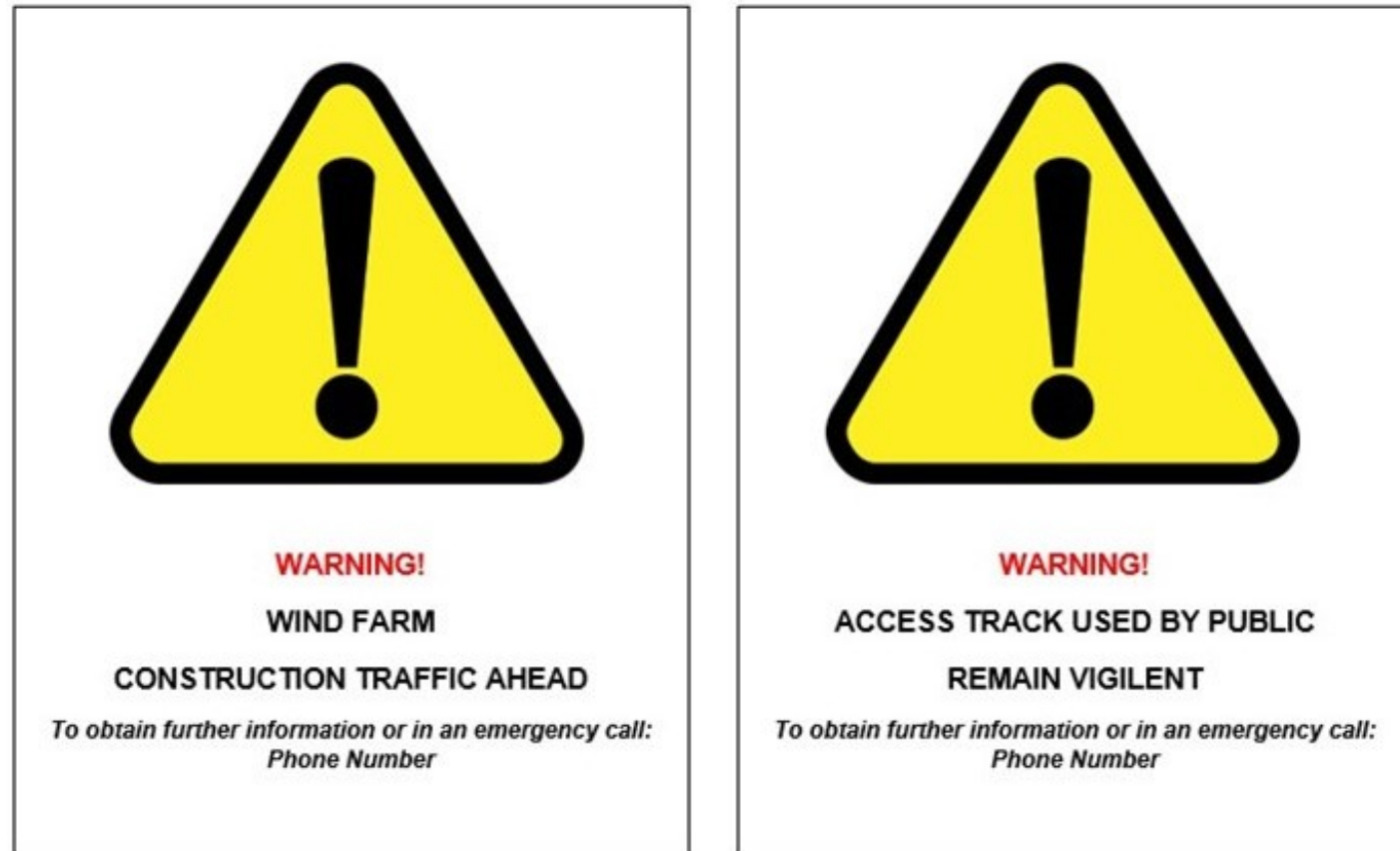
Image 13.1.3: Example of pedestrian warning sign (left) and construction staff warning sign (right) to be used along the length of the access track
