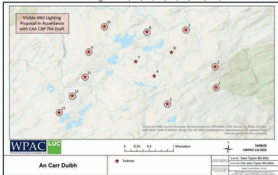
Figure 3 CAA-ANO CAP764 Compliant Lighting Arrangement
