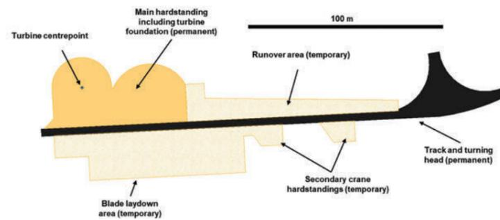
Plate 4.1 Indicative layout for turbines, hardstandings and track
