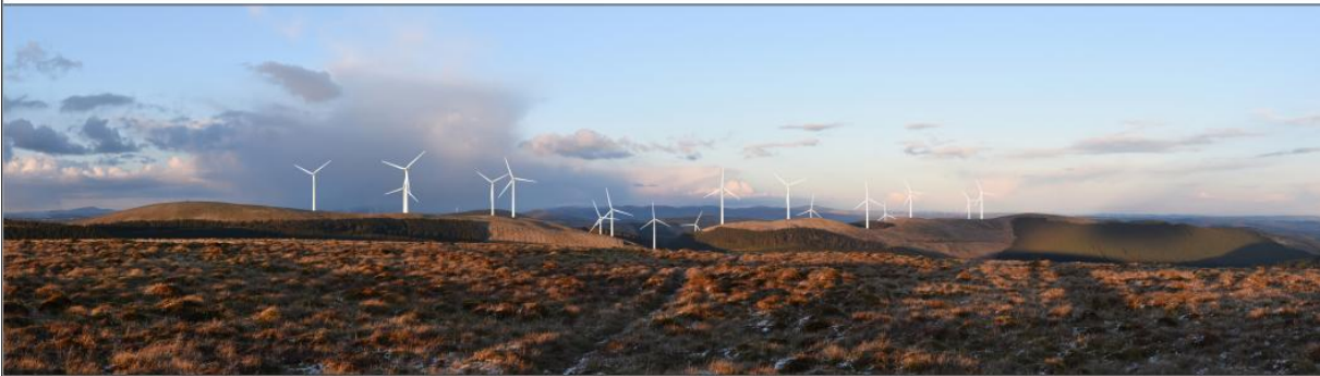
Photomontage showing current proposed layout, 17 turbines. Based on current proposal of 15 @ 230m to blade tip height and 2 @ 200m to blade tip height.
