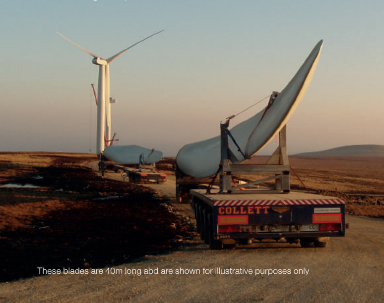
Blades being transported to Scout Moor Wind Farm
