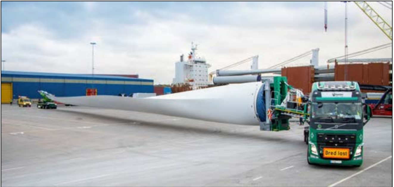
Figure 4 Indicative Blade Lifting Trailer
