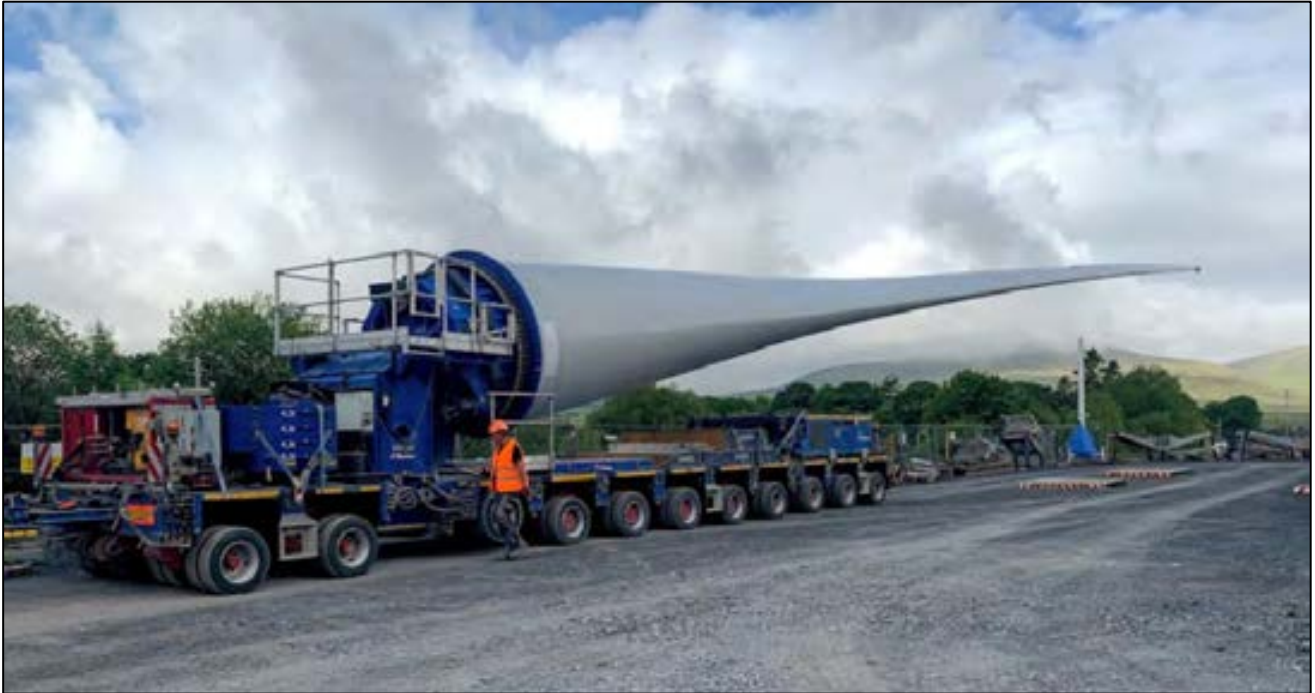
Figure 2-5: Indicative Blade Lifter Trailer
