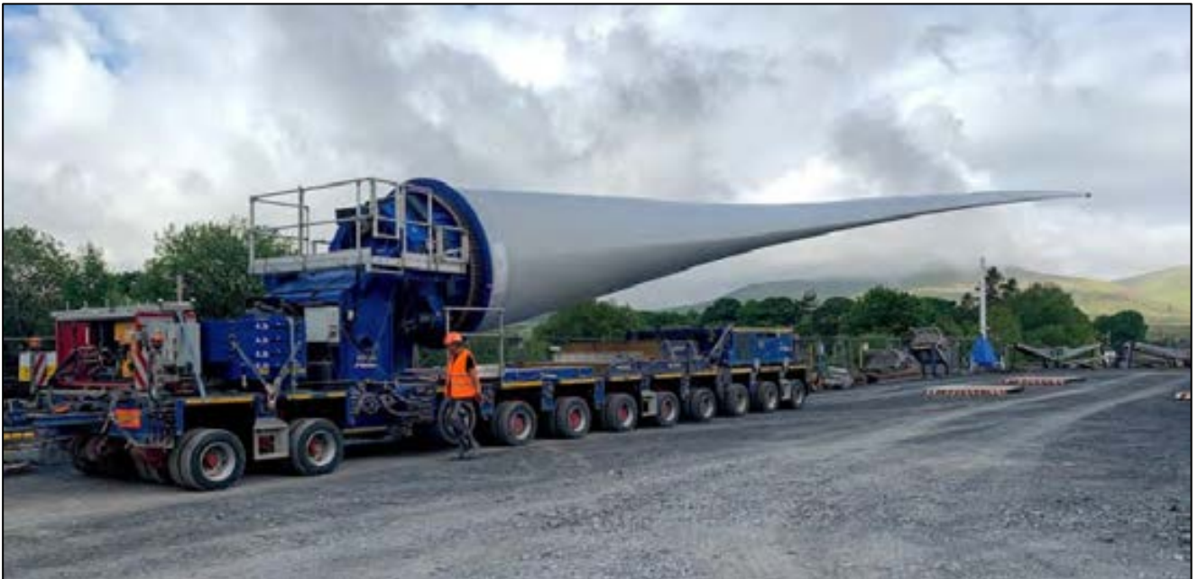
Figure 4 Indicative Blade Lifting Trailer
