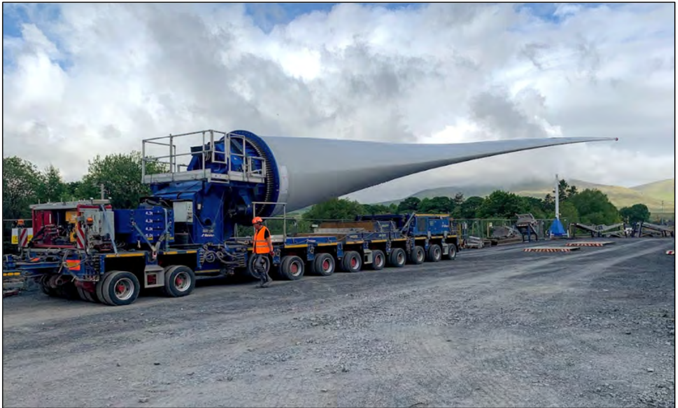
Figure 2-4: Indicative Blade Lifting Trailer
