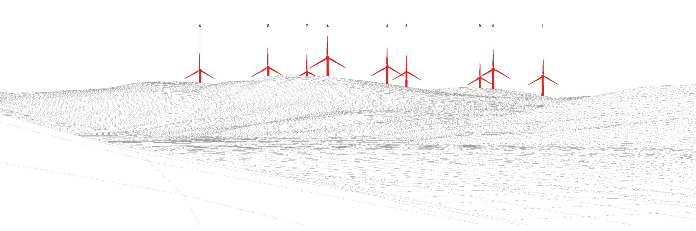
Wireframe showing submission layout9 turbines: 6 @ 200m to blade tip heightand 3 @ 180m to blade tip height.All turbines shown with a 155m rotor diameter.
