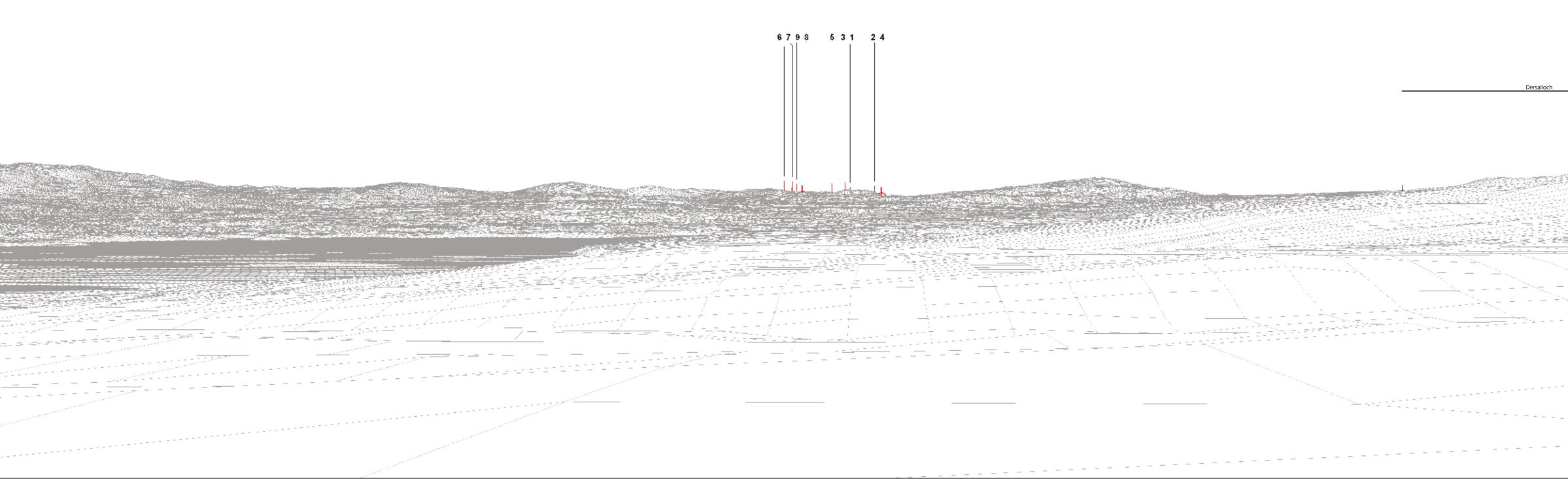
Wireframe showing submission layout 9 turbines: 6 @ 200m to blade tip height and 3@180m to blade tip height. All turbines shown with a 155m rotor diameter.
