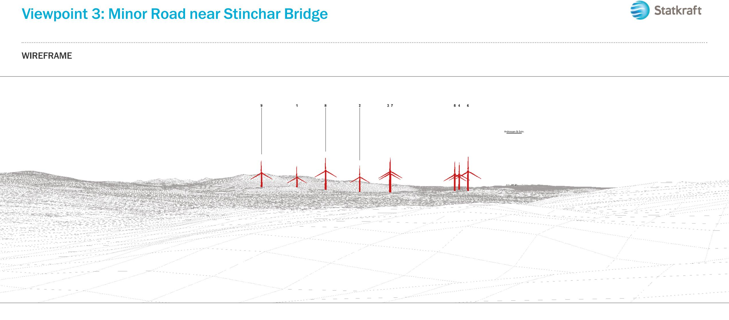
Wireframe showing submission layout 9 turbines: 6 @ 200m to blade tip height and 3@180m to blade tip height. All turbines shown with a 155m rotor diameter.
