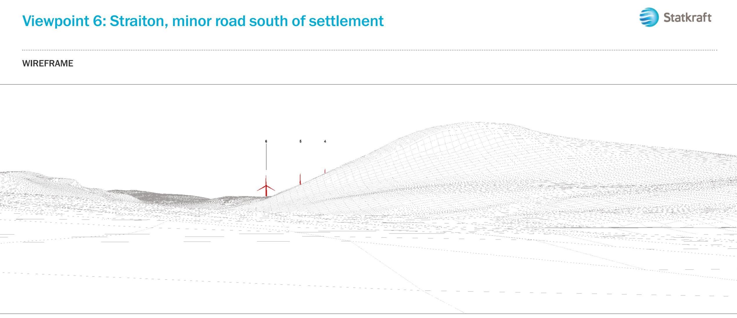
Wireframe showing submission layout 9 turbines: 6 @ 200m to blade tip height and 3@180m to blade tip height. All turbines shown with a 155m rotor diameter.
