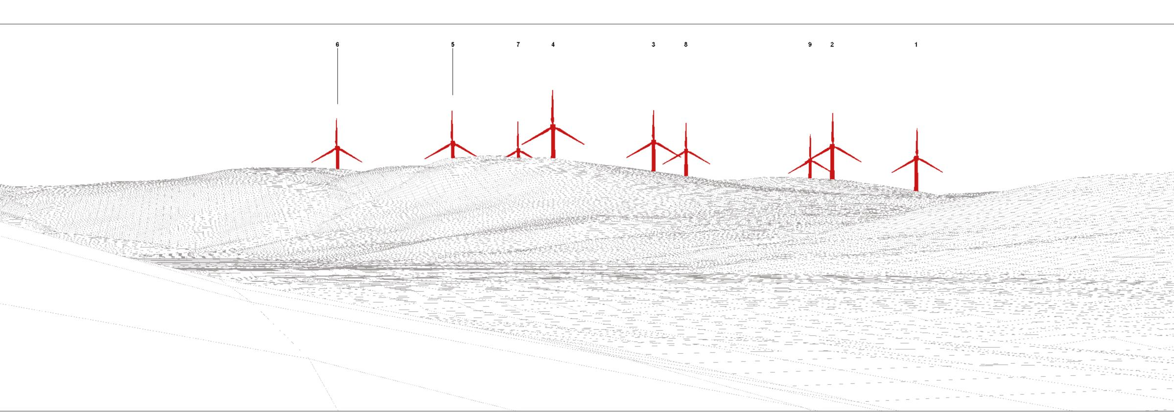
Wireframe showing submission layout9 turbines: 6 @ 200m to blade tip heightand 3 @ 180m to blade tip height.All turbines shown with a 155m rotor diameter.
