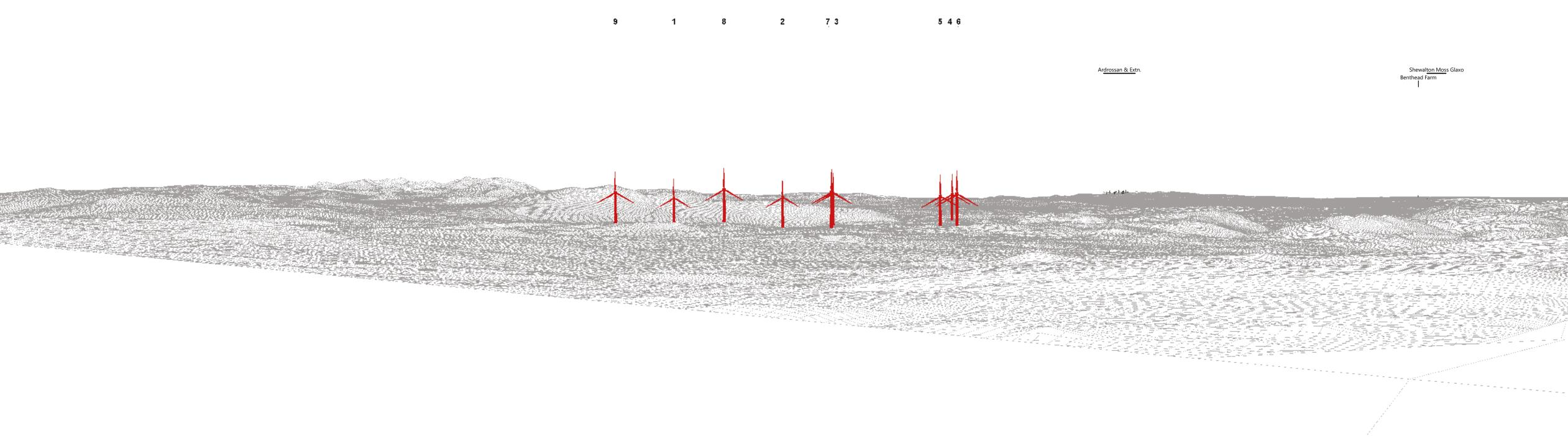
Wireframe showing submission layout 9 turbines: 6 @ 200m to blade tip height and 3@180m to blade tip height. All turbines shown with a 155m rotor diameter.
