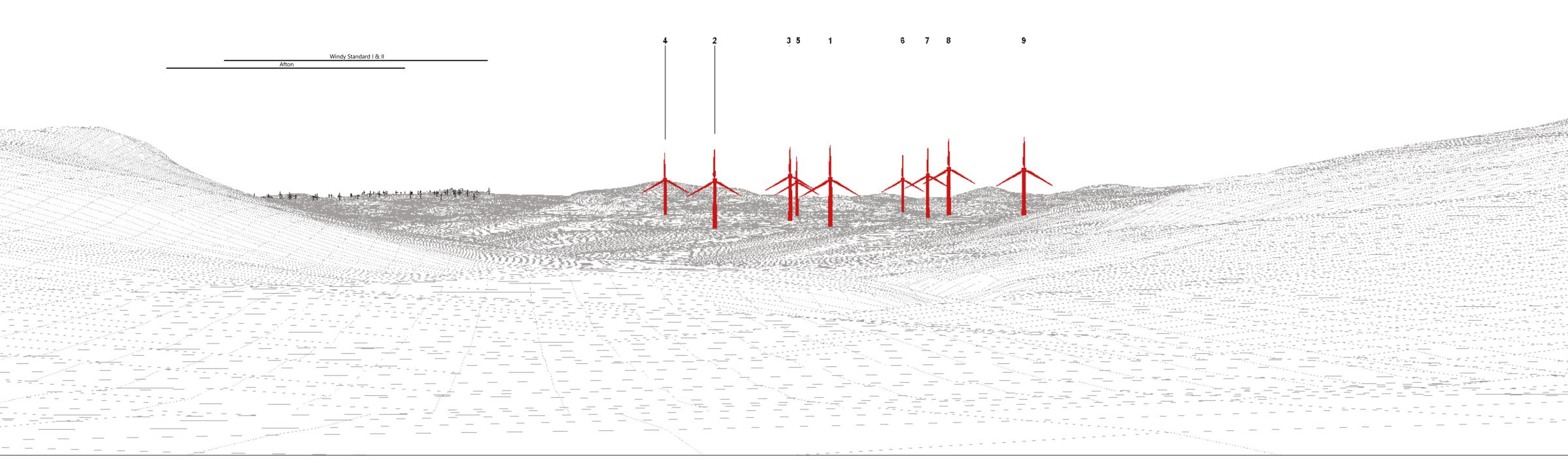
Wireframe showing submission layout9 turbines: 6 @ 200m to blade tip heightand 3 @ 180m to blade tip height.All turbines shown with a 155m rotor diameter.
