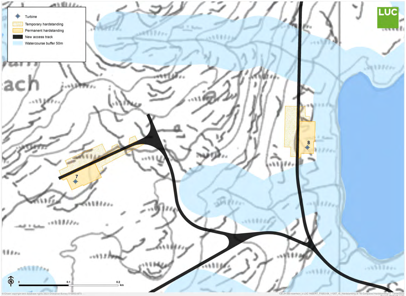
Image 4: Layout of Hardstanding at T8 Compared with Typical Hardstanding Layout at T7
