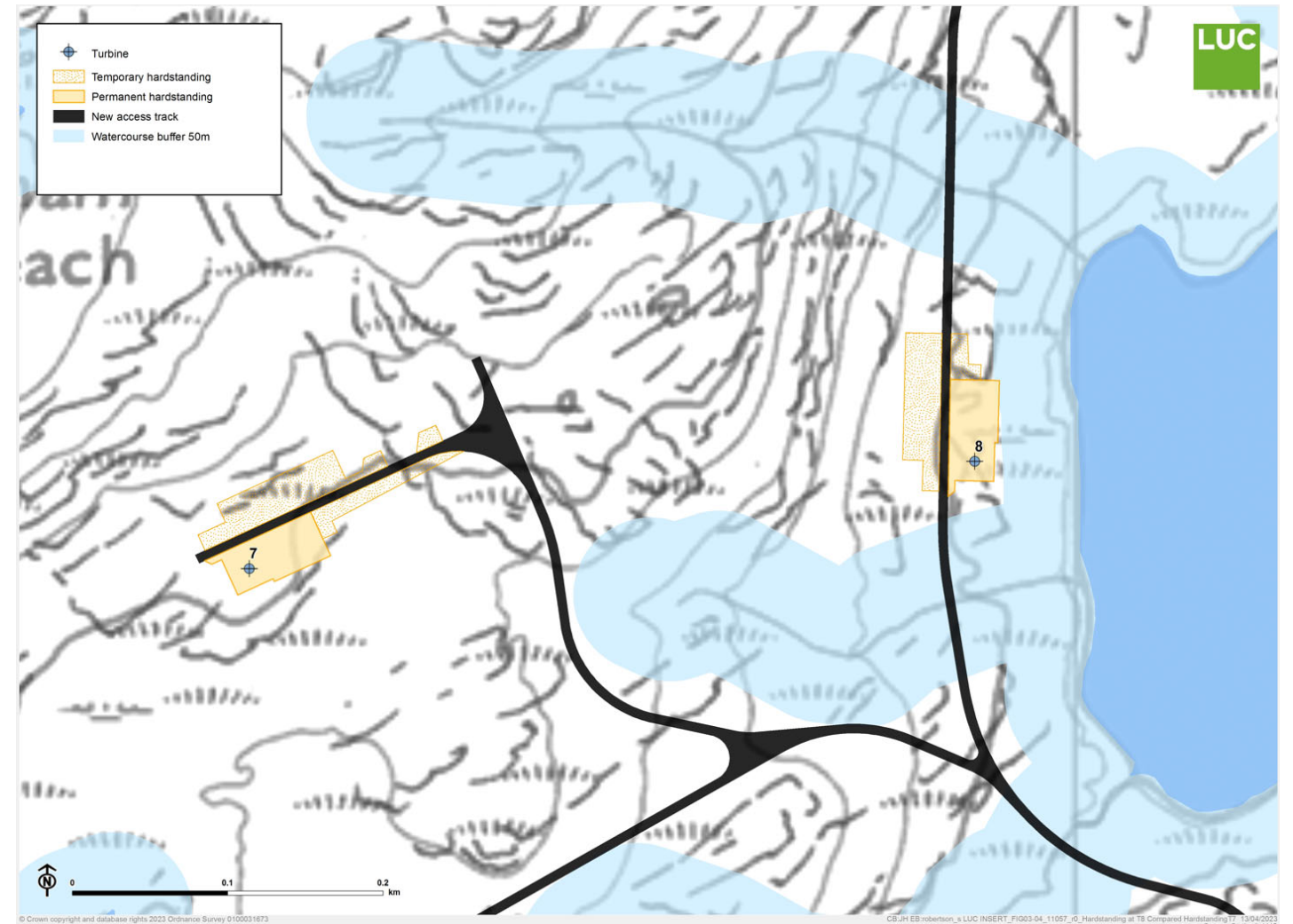
Image 3.4: Layout of Hardstanding at T8 Compared with Typical Hardstanding Layout at T7
