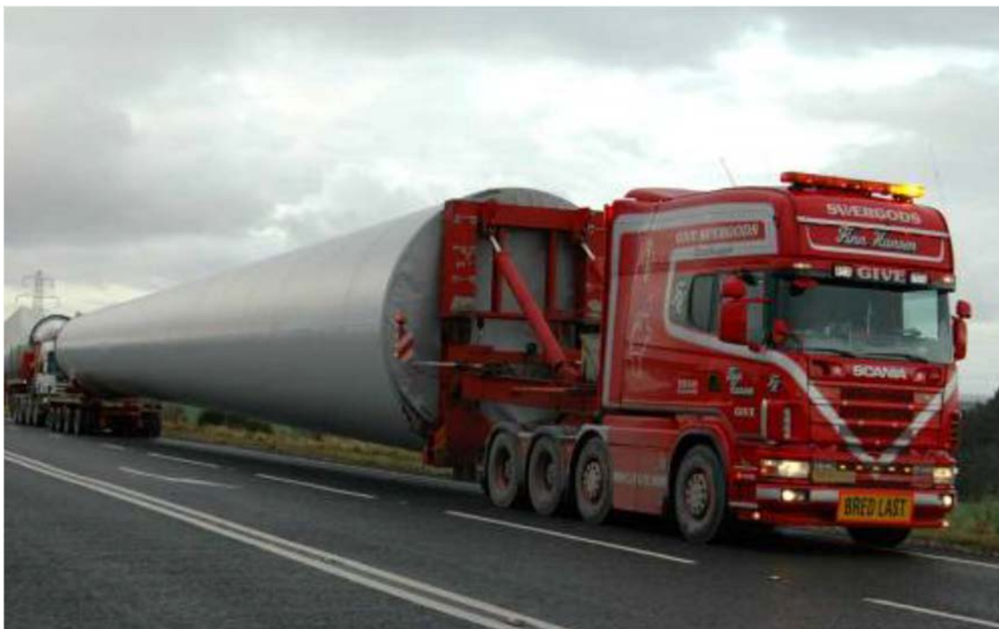
Figure 5.11: ALL Vehicle Delivering a Wind Turbine Tower Section
