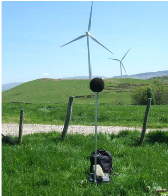
Figure 5.8: Example Background Noise Survey at an Operational Wind Farm
