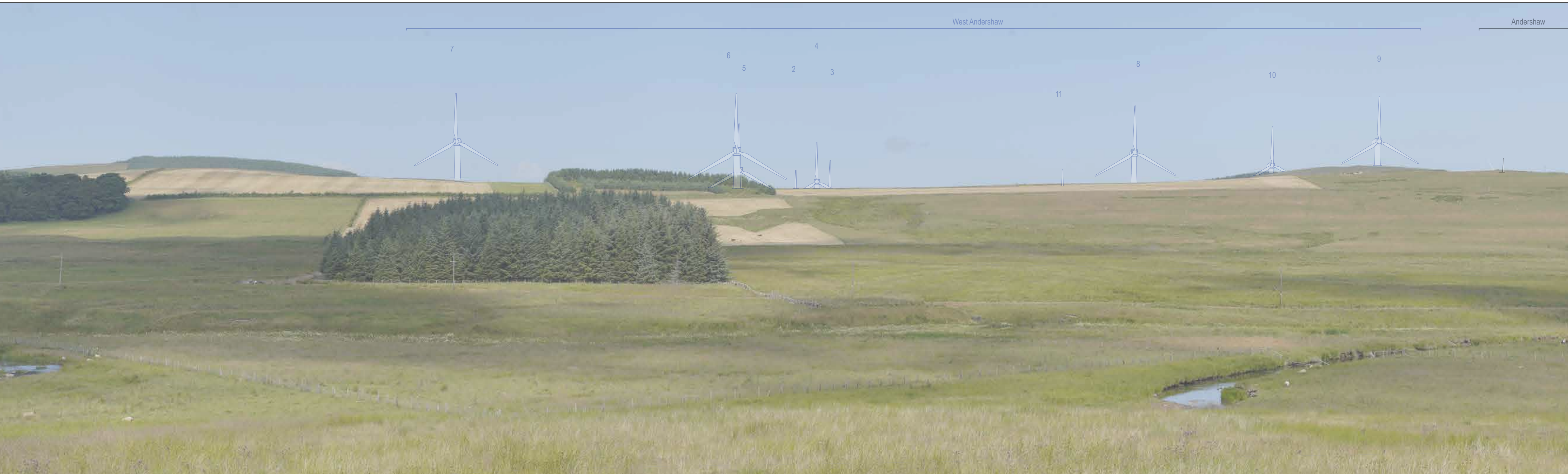
Photowireline showing proposed submission layout - 9 turbines @ 250m to blade tip height, 2 turbines @ 200m to blade tip height.
